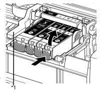
\*1 Do NOT touch the Print Head Lock Lever; remove only the ink tank.
